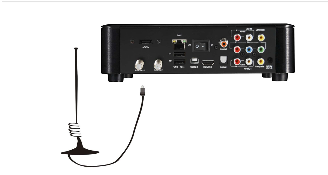
1.2.8 : DVB-T antenna connecting.
